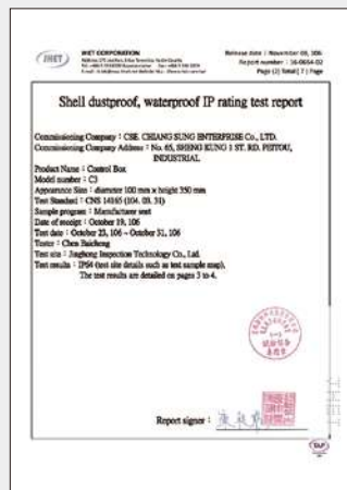
IP Test report of C3 control box
